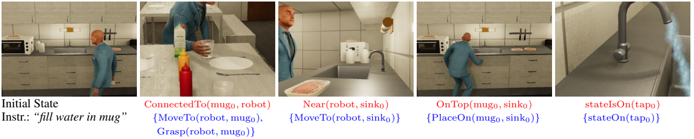
Figure 4: Sample plan in kitchen. Visualizations developed utilizing the VirtualHome Simulator (Puig et al. 2018) and a human-like agent with functionality akin to a single-arm manipulator. Predicted goal predicates shown in red. Executed plan at each time step shown in blue.
