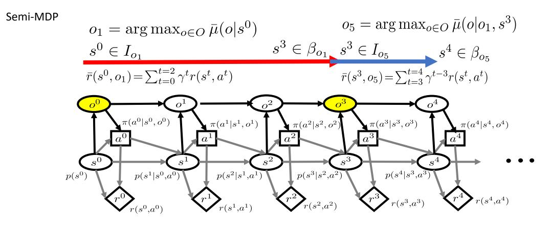
Value function for SMDP over options:  $\bar{V}^{\bar{\mu}}(s) = \sum_{o \in O} \bar{\mu}(o|s)[\bar{r}(s,o) + \gamma \sum_{s' \in S} \bar{p}(s'|s,o)\bar{V}^{\bar{\mu}}(s')]$ Sum of the probability over state transitions over option:  $\bar{p}(s'|s,o) = \sum_{j=0}^{\infty} \gamma^j p(s'=s^{t+j}|s=s^t)$ Optimal value over SMDP over options:  $\bar{V}^*(s) = \arg \max_{\bar{\mu}} \bar{V}^{\bar{\mu}}(s)$
